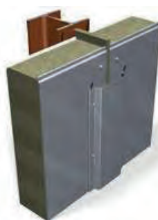
Figure 3. Linear thermal transmittance ( \Psi -value) for some basic detail solutions.
