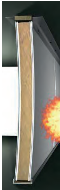
Figure 15. Behaviour of Paroc Panel System panels in case of fire.
