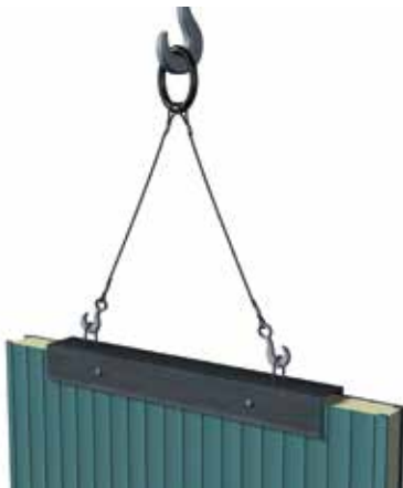
Fig. 47.: Manipulation the panel TF,TL, NC, NF (RB/RF < 7,000 mm) on a vertical lay-down ("U-carrier" – fixed by 2 pins)
