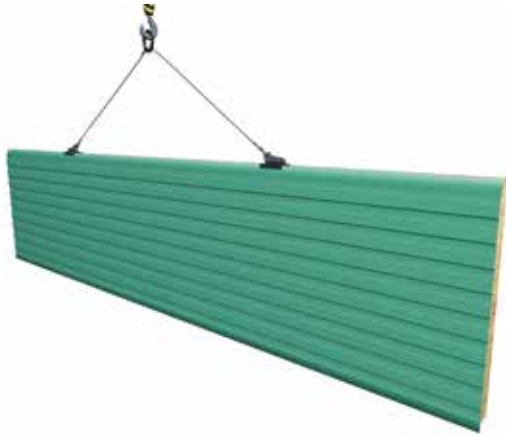
Fig. 45.: Manipulation an RF panel, on a horizontal lay-down ("Iron" – a clamp in the panel's lock – always 2 pieces at least)
