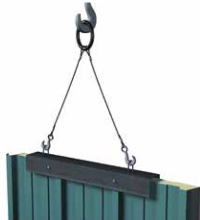
Fig. 64.: Manipulating an RW wall panel on a vertically lay-down ("U-carrier" – fixed by 2 pins)
