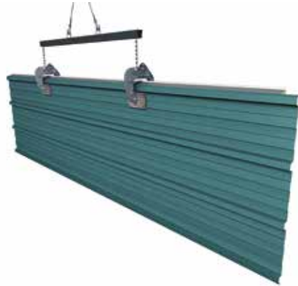
Fig. 63.: Manipulating an RW wall panel on a horizontal lay-down ("Beam tie" – for holding at a firm ridge)
