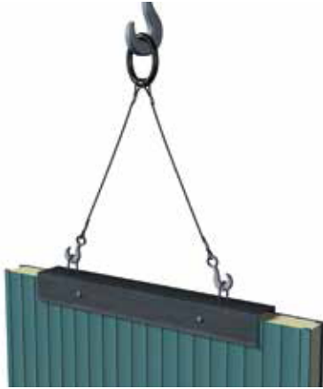
Fig. 59: Manipulation with an RH < 7,000 mm panel on a vertical lay-down. ("U -carrier" – fixed by two pins)
