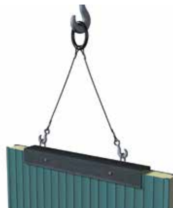
Fig. 52.: Manipulation with an AWP / AWP FLEx panel, on a vertical lay-down. (“U-carrier” fixed by two pins)
